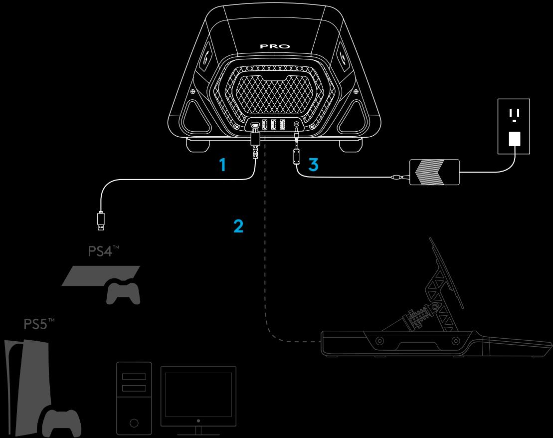
Please ensure that the power connector is fully inserted; otherwise, your PRO Wheel may not function correctly. As you insert the connector, you might feel a small click, but you can push past this until the connector is fully inserted. Do not use excessive force to insert the connector.
